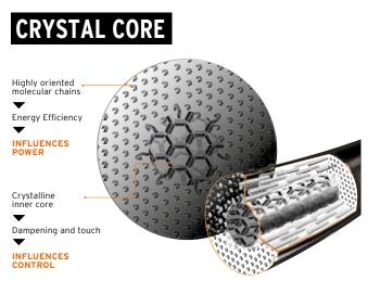
The ratio control / power is defined by the Crystal Core diameter for Hawk and Hawk Touch.
